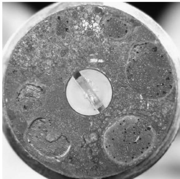
**Figure 11.** Photo of X 65 carbon steel coupon on the top of the line after 168 h of exposure in the presence of 5000 ppm total acetic acid.
